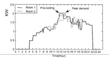
Fig. 4. Cooling power of the FAU and FCUs in two rooms.
