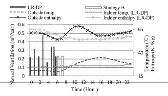
Fig. 7. Natural ventilation and relationships between outdoor temperatures and indoor temperature set points.
